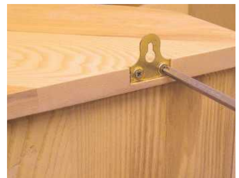
▲ Pic.22 Chisel out the recesses for the hanging plates in the rear edge of the top panel and screw the plates on
